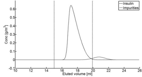
Figure 3 | The concentration profiles of the components at the end of the column. The vertical lines are the cut-off points.
