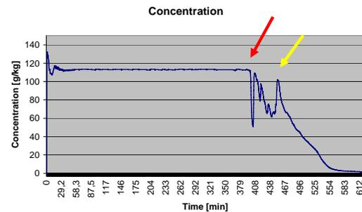
**Figure 1. Concentration in the case of a flow rate of 15 ml/min and an inlet temperature of 37 °C. Red arrow: channelling onset, yellow arrow: temporary rehomogenization of powder bed.**
