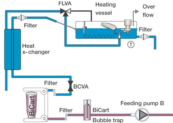
**Figure 4. Suggestion for reducing channelling. A heat exchanger may be implemented to decrease the temperature of the water to the BiCart® cartridge.**
