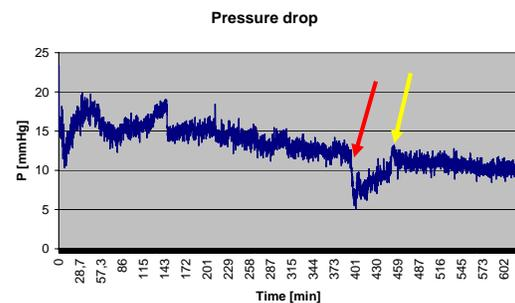
**Figure 2. Pressure drop for a test at an inlet temperature of 37 °C and a flow rate of 15 ml/min. Red arrow: channelling onset, yellow arrow: temporary rehomogenization of powder bed.**
