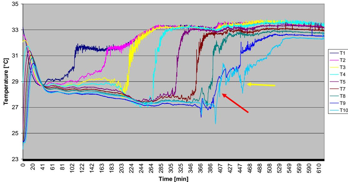
**Figure 3. Temperature profile for a test at a flow rate of 15 ml/min and a temperature of 37 °C. Red arrow: channelling onset, yellow arrow: temporary rehomogenization of powder bed.**
