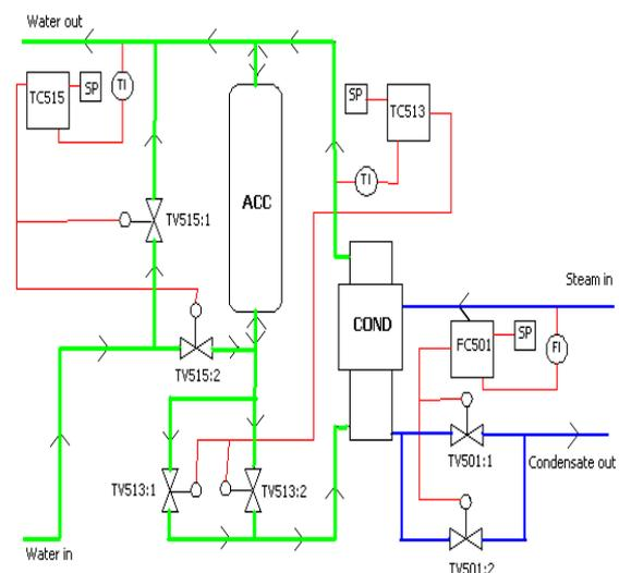
Figure 1: Sketch of the system, control loops are marked in red
