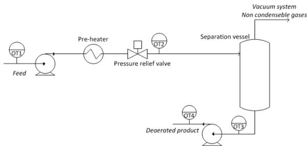
Figure 1 Schematic flowsheet of a deaeration process with oxygen sensors marked out.
