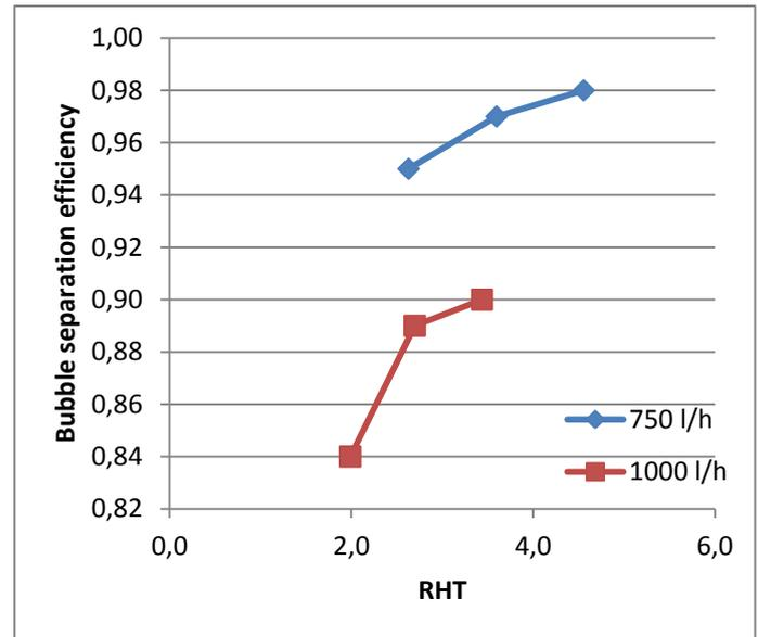
Figure 4, deaeration results in the horizontal vessel for 750 l/h and 1000 l/h.
