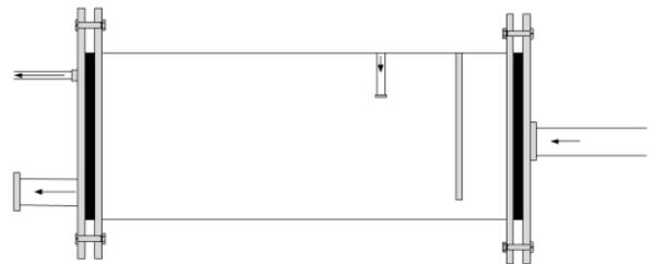
Figure 2 Schematic drawings of the two deaeration vessels.
