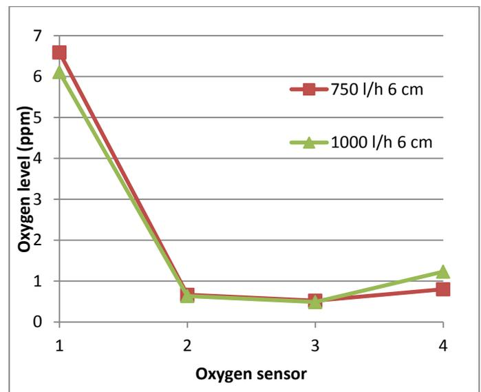
Figure 5, oxygen profile in the horizontal deaeration vessel for two flow rates at the same liquid level.
