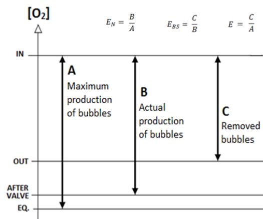
Figure 3 Picture of the separation efficiencies.
