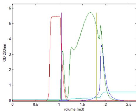
Figure 6. Optimized chromatogram for a particular cycle in the 5 recycle mode.
