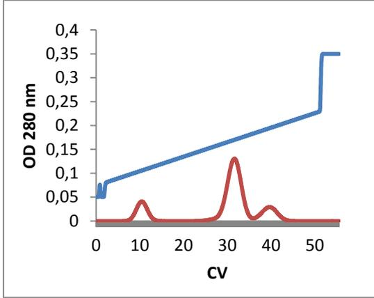
Figure 2. Chromatogram of a A,BC and D mixture for a 0.2 CV load. Di-PEGylated forms of the protein elute at lower salt concentration, followed by the mono-PEGylated and unreacted protein.
