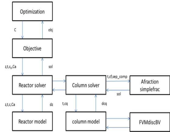
Figure 3. Function outline for the optimization. This optimization will be carried out in different case scenarios. The first will be run the simplest operation mode, the batch mode, followed by a model with 5 recycles and an infinite recycling.
