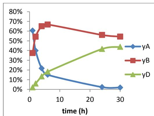
*Figure 1. Reaction yields for components A, B and D with 1.5 substrate molar ratio and 10g/l of initial native protein concentration.*
